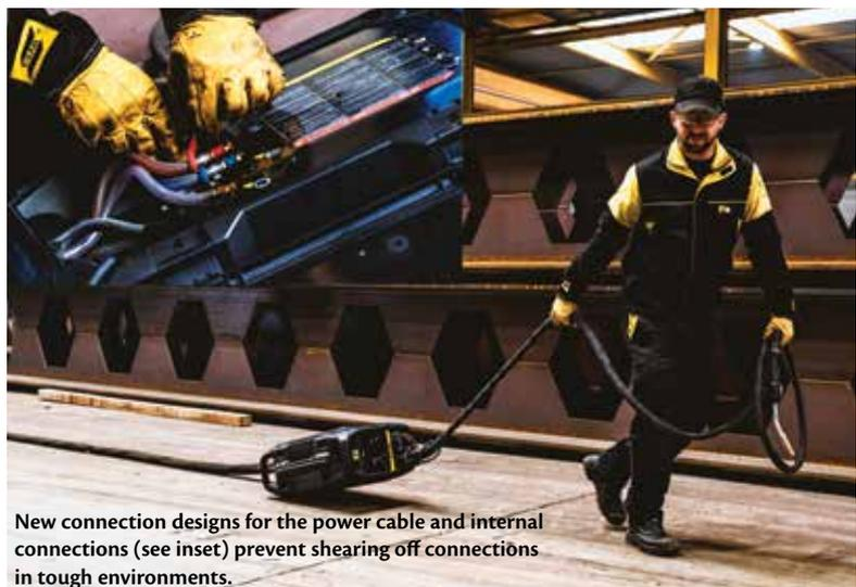
New connection designs for the power cable and internal connections (see inset) prevent shearing off connections in tough environments.
