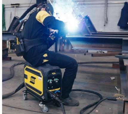
The optional wheel kit mounts in the vertical orientation shown here or in a horizontal position for greater stability and to slide under weldments.
