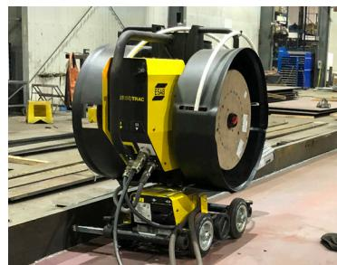
Versotrac enables orienting the welding head for fillet or butt welds and the flexibility to quickly adapt to different beam configurations. The PEK controller communicates more welding & process data, improving traceability.
