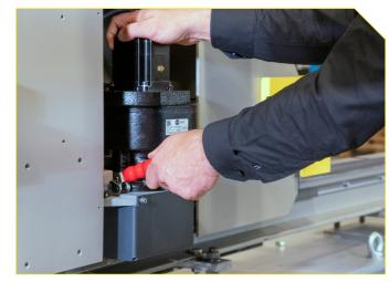
The Combirex PRO is equipped with a heavy-duty crane rail to ensure accurate motion and long machine life. A new quick-disengage mechanism for the X-axis drives improves serviceability to reduce down-time. The machine's new side carriage design allows faster drive speeds and improved stability.
